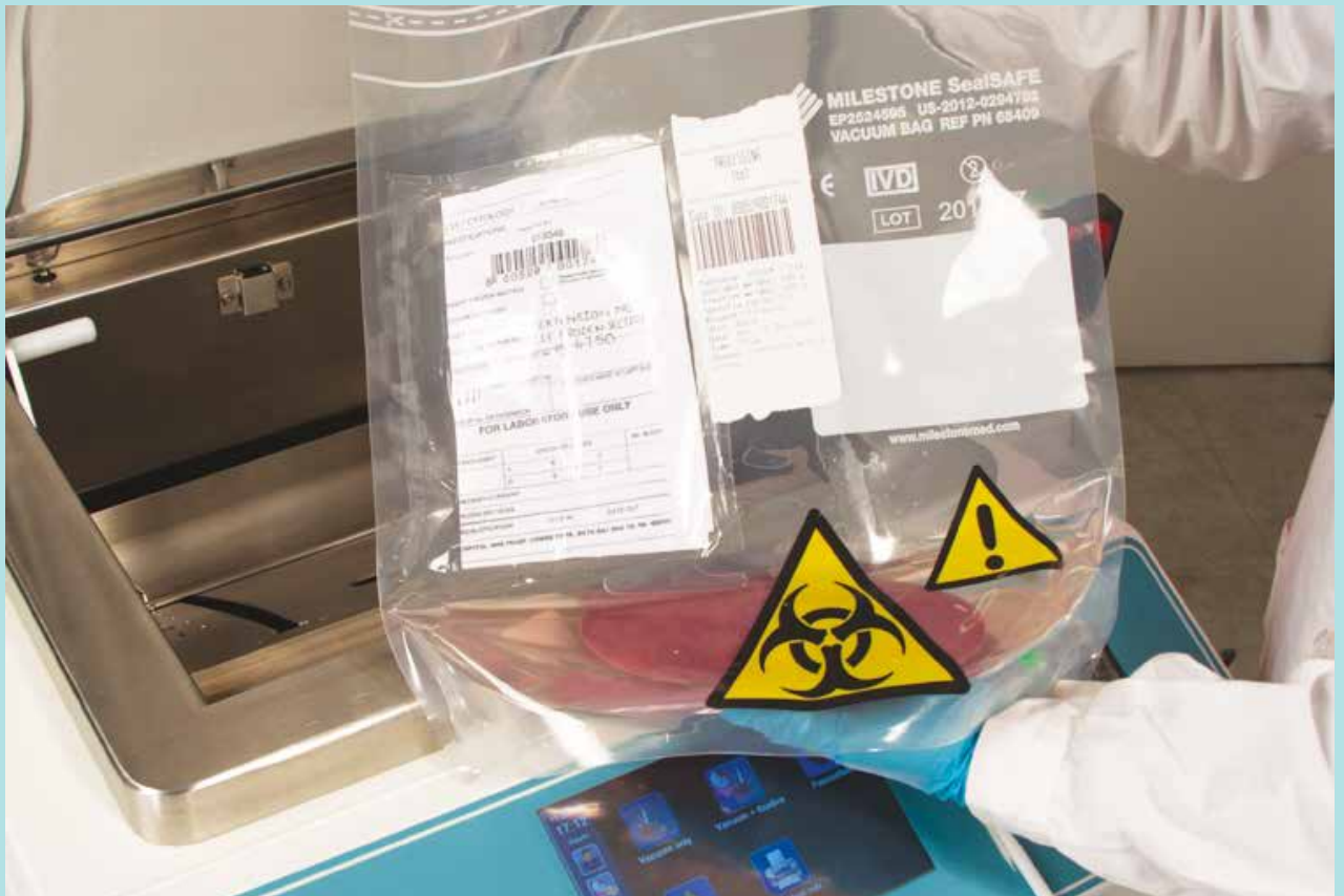
SealSAFE - Biospecimen vacuum sealing plus automated fixative addition
