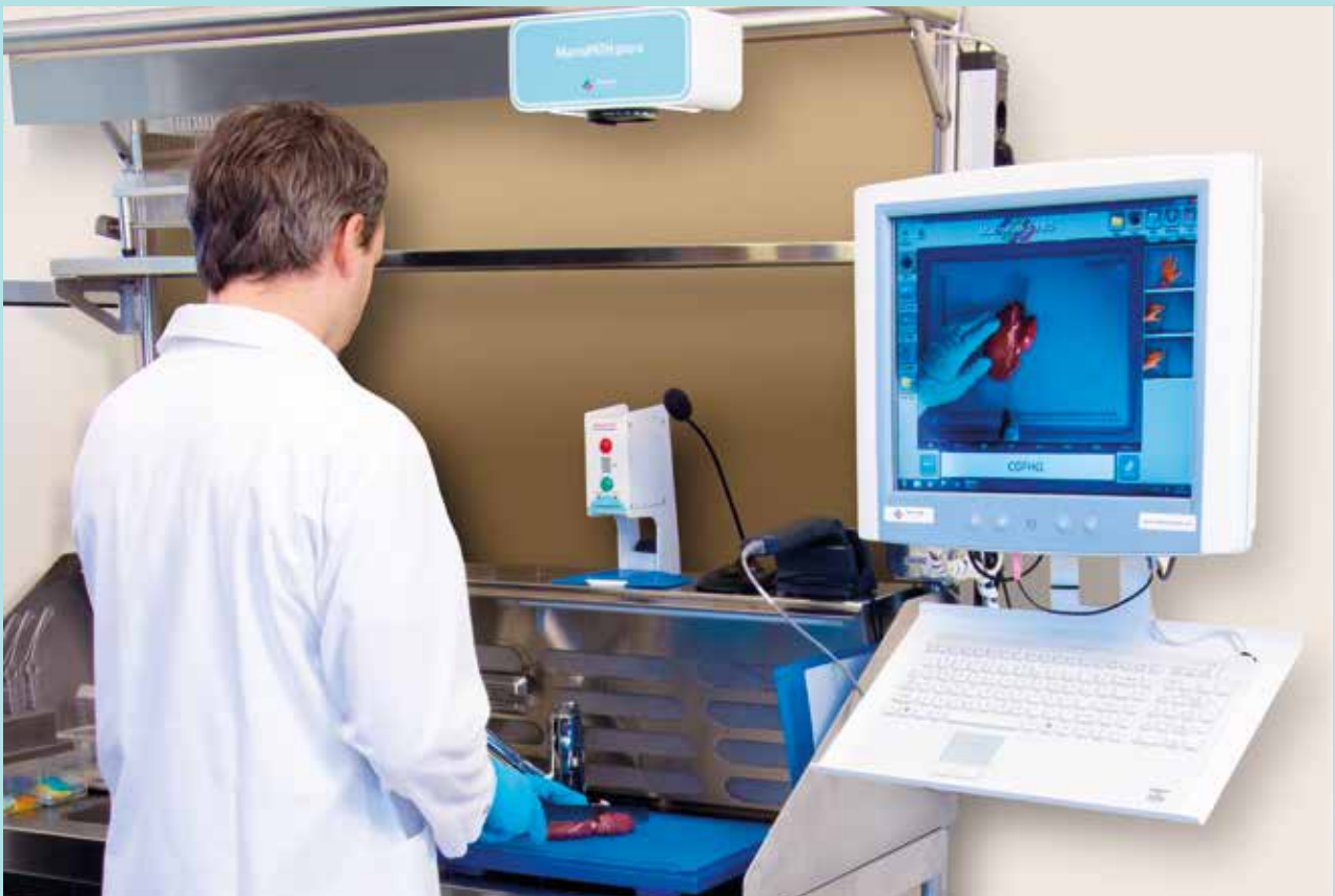
MacroPATH - Macro digital imaging system for the grossing room
